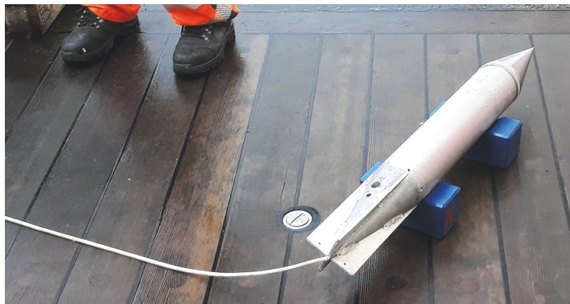
Figure 13: Thy dynamic free-fall penetrometer Nimrod (Stark, 2010) onboard R/V Heincke during expedition HE544 (Holler and Bruns, 2020).
