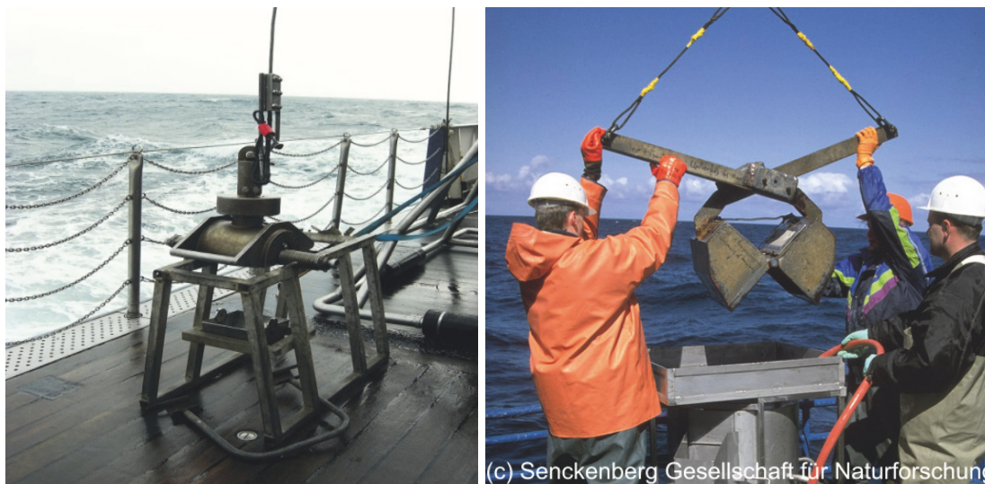
Figure 12: Two different devices to obtain surface sediment samples were used during the field work of this thesis. Left panel: The Shipek-grab onboard R/V Alkor. Right panel: The Van Veen grab onboard R/V Senckenberg.
